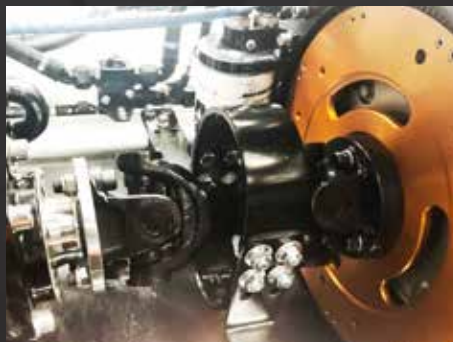
Client: Sprintec Description: Adventure Tourism Jetboat 0-100kph in 2.5 seconds Engine: Custom LS3 (615hp) Driveshaft: Turret 1400 series
