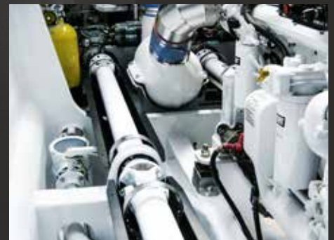
Ship: 22m High Speed Catamaran Description: 4 x Water jets Engine: 4 x 750hp CAT Driveshaft: 4 x Turret 17 series
